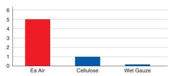
AMSOIL Ea Motorcycle Air Filter media removes 5 times more dust than traditional cellulose filters and 50 times more dust than wet gauze.
